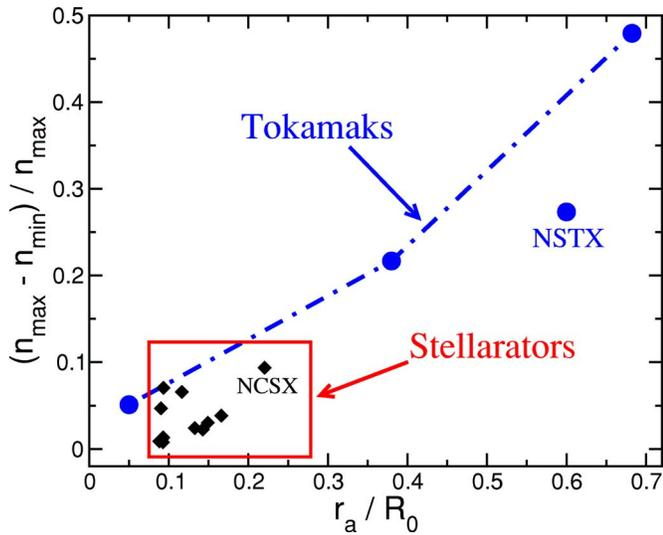
FIG. 11. (Color online) Peaking factor  $(n_{\max} - n_{\min})/n_{\max}$  as a function of inverse aspect ratio, both tokamak and stellarator results. Note that a large-aspect-ratio tokamak (inverse aspect ratio  $\epsilon=0.05$ ) with circular unshifted flux surfaces has been considered in addition to the cases described in the text.
