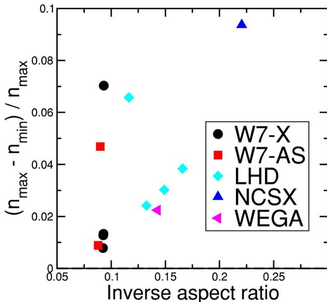
FIG. 12. (Color online) Peaking factor  $(n_{\max} - n_{\min})/n_{\max}$  as a function of inverse aspect ratio, stellarator results. Note that for a classical  $l=2$  stellarator WEGA (Ref. 24), the LHD configurations with  $R_{\text{ax}}=4.05$  and 3.90 m, low- and high-mirror W7-X configurations have been considered in addition to the stellarators described in Sec. IV.
