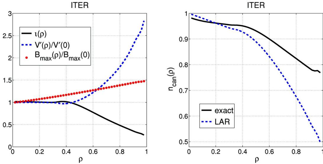
FIG. 1. (Color online) ITER (inverse aspect ratio  $\epsilon \approx 0.38$ ). Left: Rotational transform  $\iota$ , normalized flux derivative of the magnetic volume ( $V' = dV/d\psi$ , where  $\psi$  is the poloidal flux), normalized maximal magnetic field on a surface  $B_{\max}$  as functions of  $\rho = \sqrt{\chi/\chi_a}$  with  $\chi$  being toroidal flux. Right: Canonical density computed using Eq. (15) (solid line) vs large-aspect-ratio limit given by Eq. (19) (dashed line).
